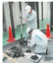
Core Drawing Operation for Heavy Metal Survey at Okaya Site
