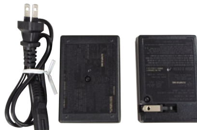
Reducing power cord weight: An old-type product is shown on the left and a new product with a built-in plug on the right.
