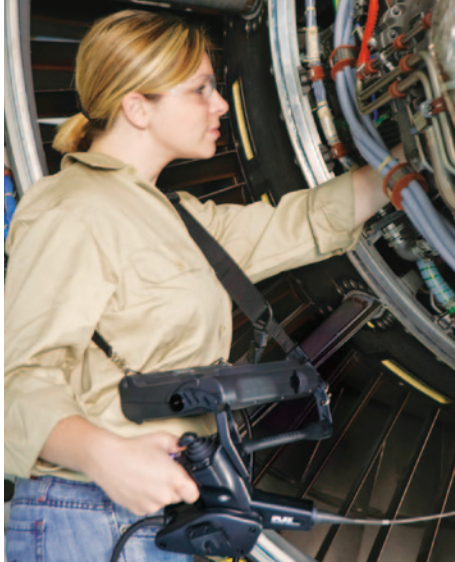
Inspecting an engine with an industrial endoscope
