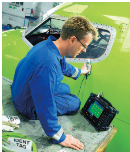
Inspecting the area around an aircraft fuselage with an eddy current array flaw detector
