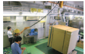
Packaging is subjected to a dropping test.
